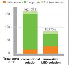
The aforementioned figures are based on an observation period of 15 years, an illumination time of 8,760 hours (continuous) and energy costs of 0.14  $\in$  per kWh.The comparison lamp was a conventional T5 fluorescent light with a system output of 54 W and 59.6 W.
